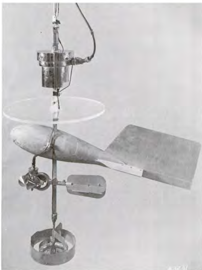
Fig. 4. Instrument string for water sampling and current measurements
